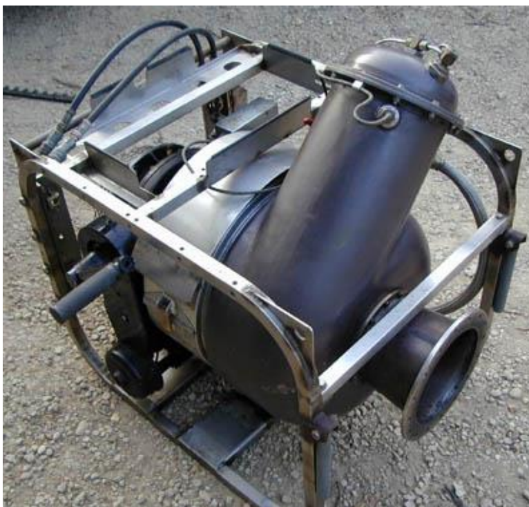
100HP hand-crank stationary gas turbine (Deutz T216)
