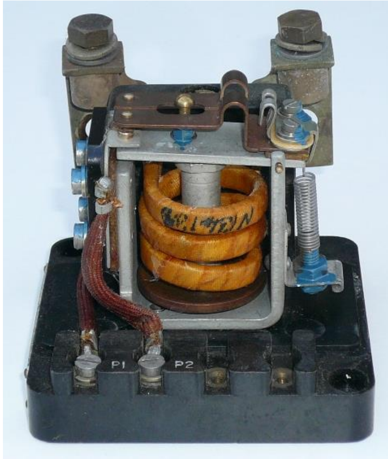
Starter circuit under-current relay
