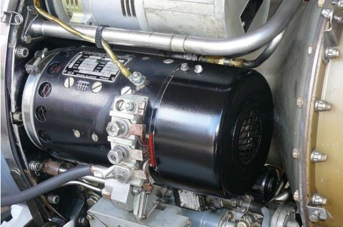
DC starter generator fitted to gas turbine engine (Turbomeca Astazou)
